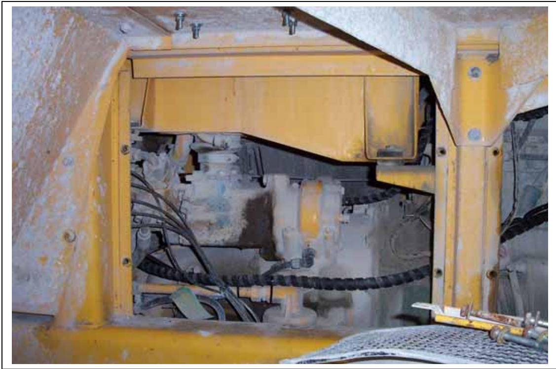
Hoses continuing forward on engine towards the evaporator.
