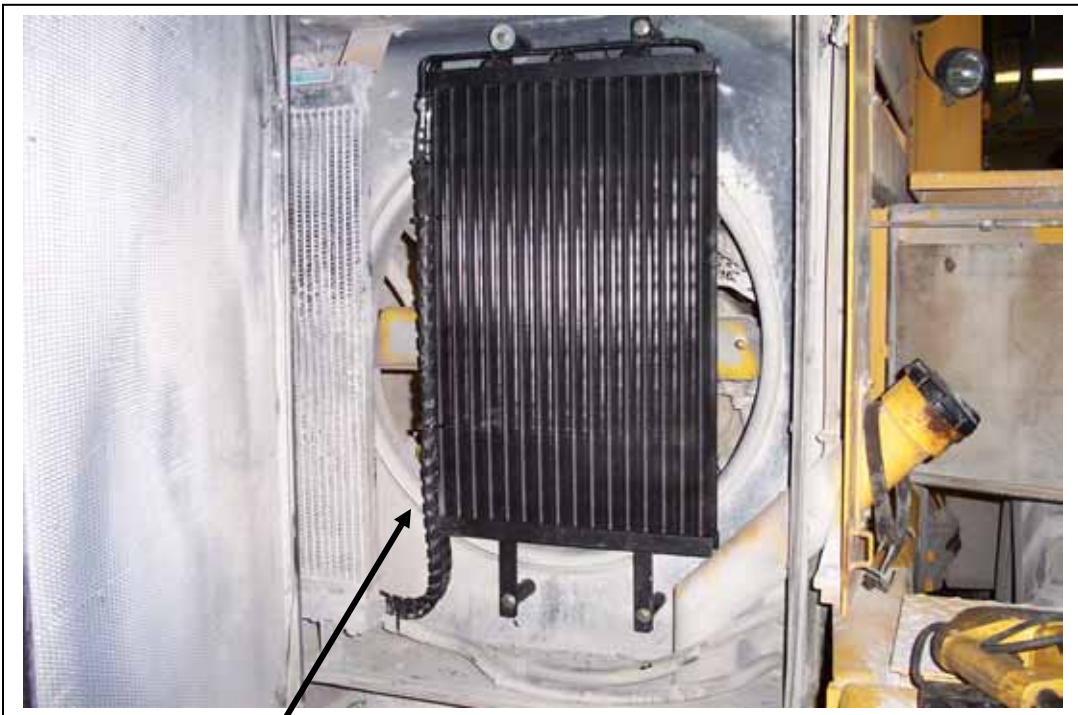
Holes marked and drilled for 3/8" bolts to mount the condenser frame.
