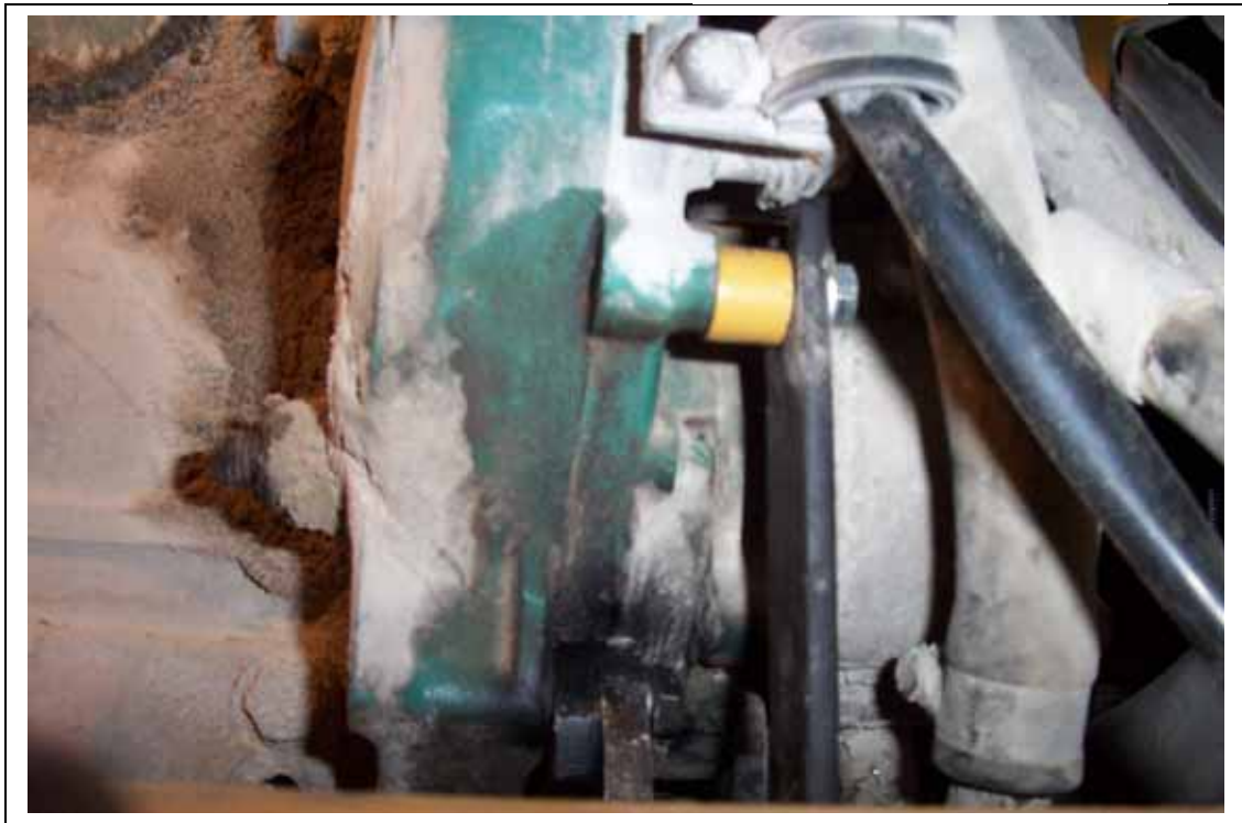
Stiffener bracket . Cut to length and bolted to engine using a M8 x 40 MM bolt.
