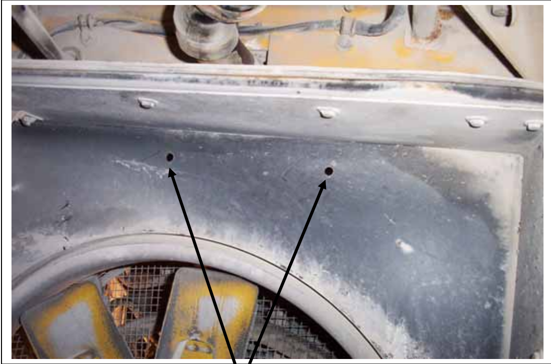
Holes marked and drilled for 3/8" bolts to mount the condenser frame.
